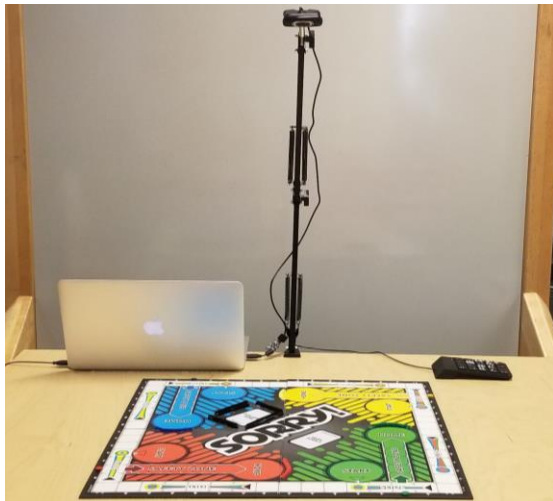
Figure 2. System setup that shows the laptop, webcam, numeric keypad, and game board.
