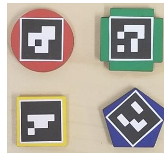
Figure 3. Wooden game pieces that have been laser cut into the shape of circles, squares, and pentagons with ArUco markers on them.
